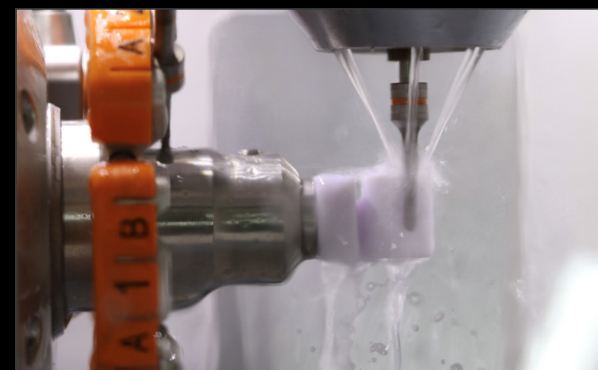
Chairside milling lithium disilicate block.
