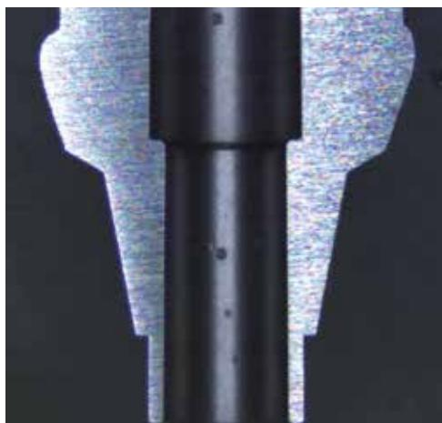
Cross section through a CoCr abutment after casting on with a non-precious-metal alloy.
