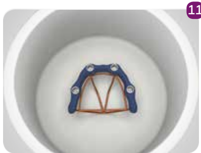
Castable ring with waxed framework.
