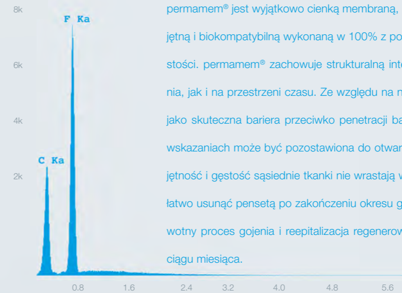
Energy-dispersive X-ray spectroscopy (EDX) of permamem®: molecular fingerprint. Characteristic peaks of carbon and fluorine. No other phases detectable.
