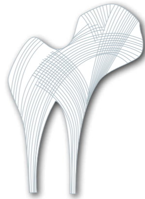
Wolff's law – bone density and structure adapt to changes in load
