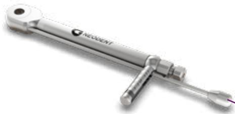
Neodent® Torque Wrenches are demountable because they need to be cleaned internally before the sterilization process in the autoclave. The thin rod is used to measure and indicate the torque value when handled.
