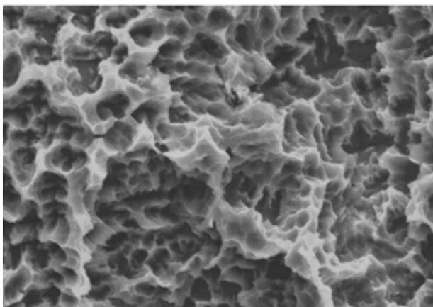
FIGURE 9. Micro (0.3 - 1.3 μm) and macro (15 - 30 μm) roughness for Acqua and NeoPoros.
