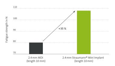
Source: data on file, according to ISO 14801, conditions 2016 Straumann® Mini Implants, made from Roxolid® show a 35% higher fatigue strength than competitor mini implants.
