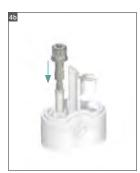
Step 4 – Attach the transfer piece to the implant
