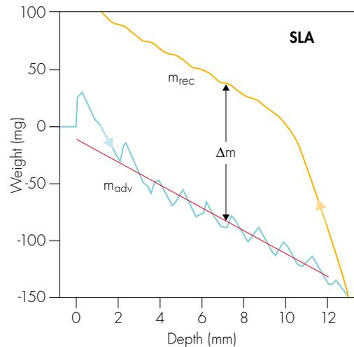
Fig. 1: Wilhelmy Force loop for SLA, showing hysteresis ( $\Delta m$ ).
