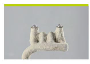
**Step 5 – Casting and devestment** Cast the bridge framework.
