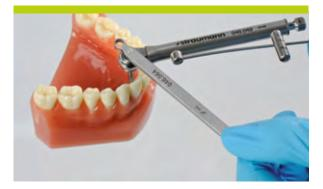
Place it on the implants and tighten the screw between 15 Ncm and 35 Ncm (depending on implant stability) using the SCS screwdriver along with the ratchet and the torque control device.
