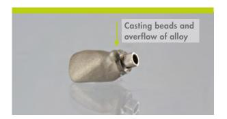
**3.** Extruded casting metals and casting pearls cannot be removed from the connection part of the gold abutment.
