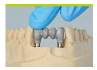
Assess tension-free fitting on the master cast (Sheffield test).
